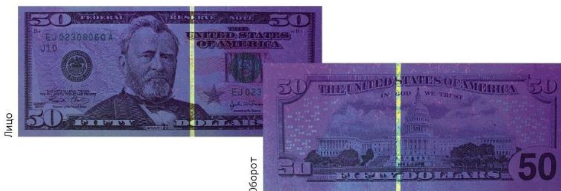
14. Rasm. Yashirin xususiyatlarga ega bo‘lgan himoya ipi (ultrabinafsha nurlanish ta‘sirida lyuminestsent).
